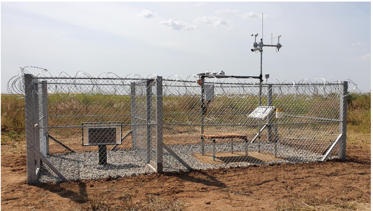
Figure 1: Soroti on-site solar and meteorological measurement station
