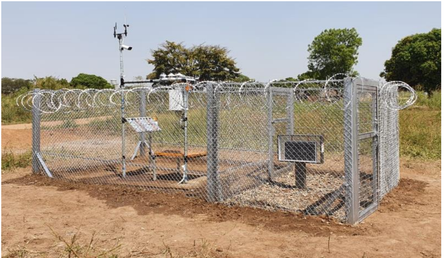
Figure 1: Wadelai on-site solar and meteorological measurement station
