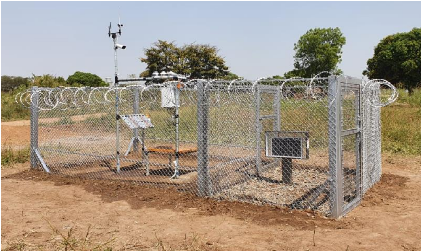
Figure 1: Wadelai on-site solar and meteorological measurement station
