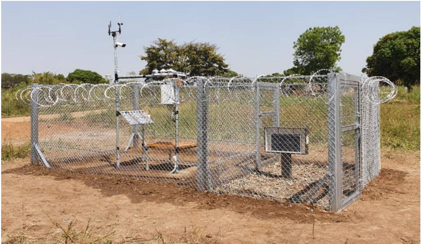
Figure 1: Wadelai on-site solar and meteorological measurement station
