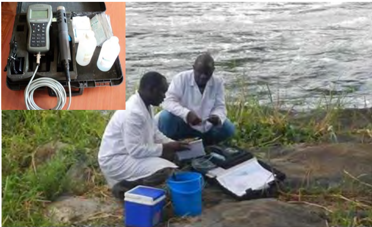
Photo 1: Onsite water quality measurements on the Victoria Nile at Nampanyi Village using the multi-parameter field water meter (HANNA HI 9828)
