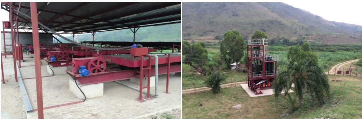
Figure 53: Shaking tables (left) and spiral concentrator (right) installed at Isingiro Tin Mine Project
