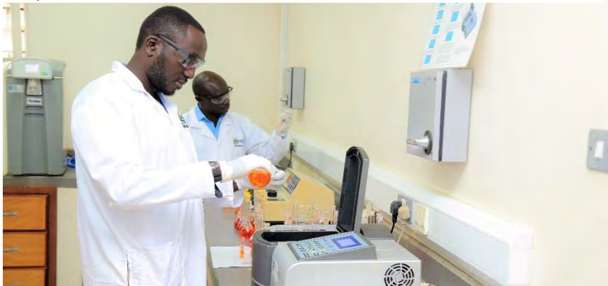
Picture 24: Henry Onyeye, Senior Chemist using the Ultra Violet- Visible Spectrometer for qualitative and quantitative analysis of minerals, rocks and ore.
