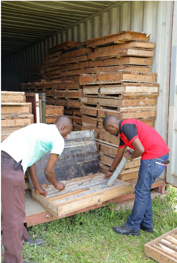
Picture 20: Drill Cores for Mineral Sampling
